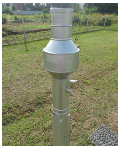
Gambar 4. Penakar Hujan Manual Ombrometer
